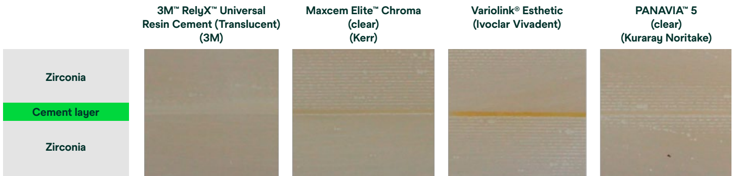
Fig. 14: Discoloration of cement layers after 24 hours of storage in coffee solution. Source: 3M internal data
