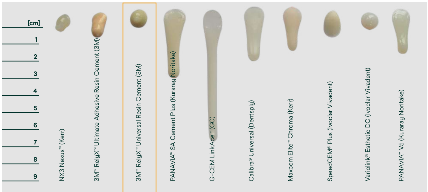
Fig. 2: To compare the flow properties, equal amounts of each cement were applied on a pad which was stored upright at 36°C/96.8°C for 2 minutes before the cement was light-cured.
