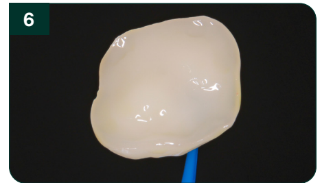
Bonding surface after HF etching and priming with 3M ™ Scotchbond ™ Universal Plus Adhesive.
