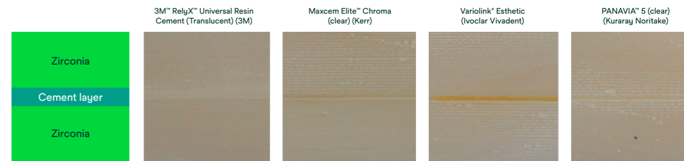
Fig. 14: Discolouration of cement layers after 24 hours of storage in coffee solution. Source: 3M internal data
