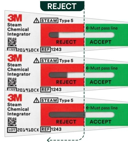
The color bar is in the **REJECT** window, indicating that the necessary conditions for sterilization have not been met. The pack should be reprocessed and the cause of sterilization failure should be investigated. **If the color bar is in the REJECT region or on the line, it is considered a fail.**
