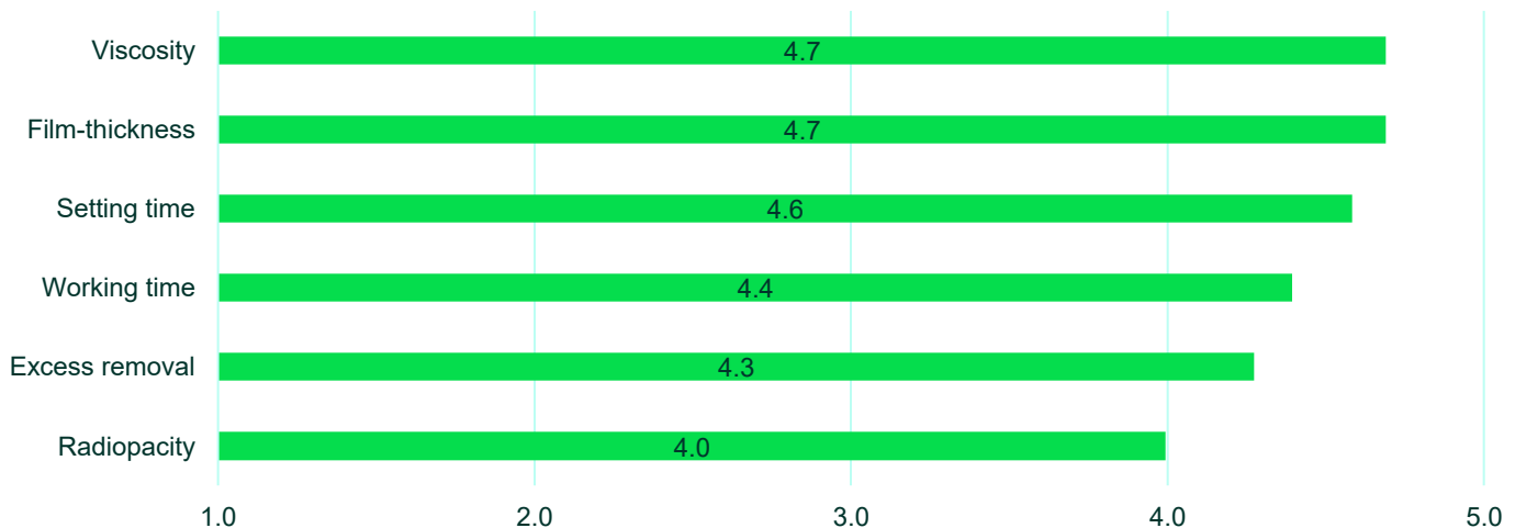
Figure 23: Average rating of key attributes of RelyX Universal Resin Cement on a five-point scale (1= poor, 2= fair, 3= good, 4= very good, 5= excellent).
